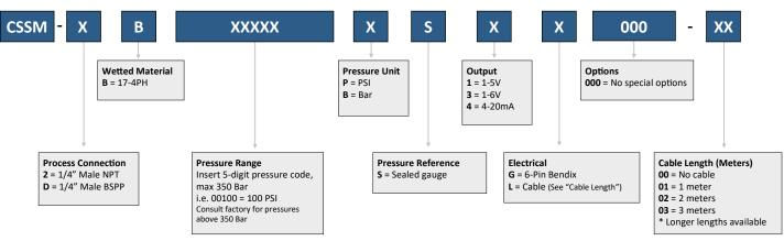
Ordering Example: CSSM-2B01000PS4G000-00 (1/4" Male NPT, 17-4PH, 0-1000 PSI sealed gauge, 4-20mA, 6-Pin Bendix)
