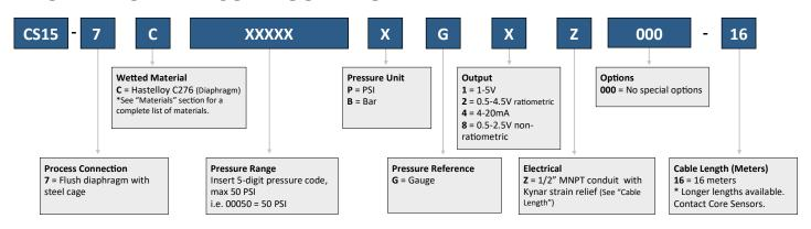
Ordering Example: CS15-7C00010PG4Z000-16 (Steel cage, Hastelloy C276, 0-10 PSI gauge, 4-20mA, 1/2" MNPT conduit w/ Kynar strain relief, 16 meter cable)
