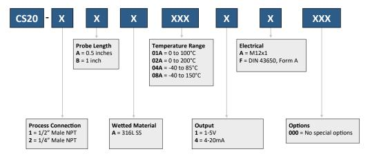
Ordering Example: CS20-2BA01A4A000 (1/4" Male NPT, 1 inch probe, 316L SS, 0 to 100°C, 4-20mA, M12x1)
