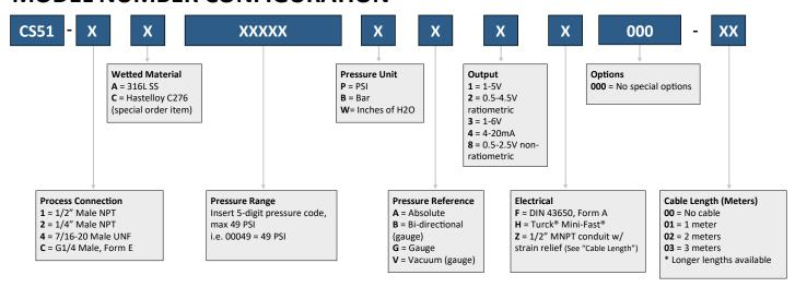
Ordering Example: CS51-2A00010PG4H000-00 (1/4" Male NPT, 316L SS, 0-10 PSI gauge, 4-20mA, Turck® Mini-Fast®)
