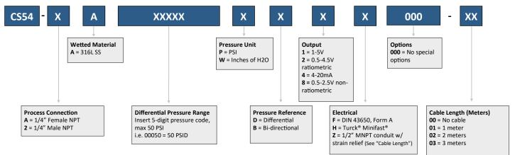
Ordering Example: CS54-AA00010PD4H000-00 (1/4" Female NPT, 316L SS, 0-10 PSI differential, 4-20mA, Turck<sup>®</sup> Minifast<sup>®</sup>) Not all configurations are available. Our sales team can recommend the closest available configuration based on your requirements. Contact Core Sensors for configurations not shown. Visit our <u>How To Buy</u> page or <u>contact us</u> for a quote.
