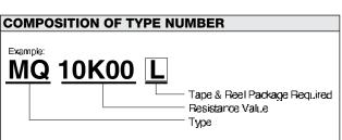
Resistance value, in ohm, is expressed by a series of five characters, four of which represent significant digits. R or K is a dual-purpose letter that designates both the value range (R for ohmic; K for kilo-ohm) and the location of the decimal point.
